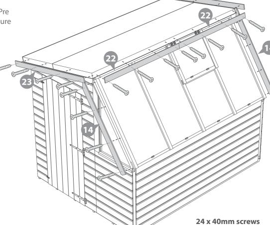
Fix Cover trims using 30mm screws as shown. Pre drill holes to avoid splitting.
