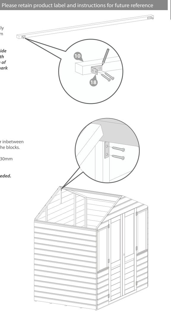
\*Measure 67mm from each side of the ridge bar and mark with a pencil. Align the front edge of the bracket with the pencil mark as shown in the illustration.
