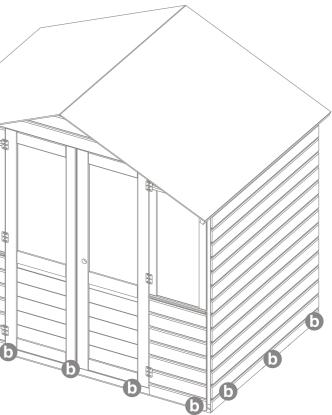
Fit the angled fascia block to the apex of the roofs, making sure it is flush with the roof sheet, securing in place with 4x40mm screws.
