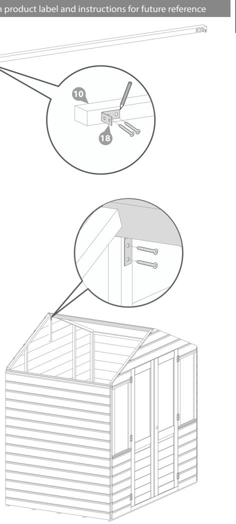
Fix an eaves frame to the edge of each roof sheet with 5x30mm screws per frame.
