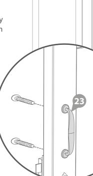
Fix the presslock to the inside of the master door, making sure to align the barrel and the key hole.
