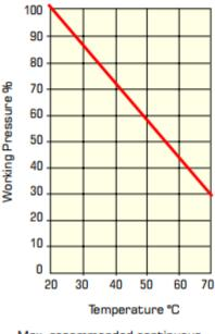
Max. recommended continuous working temperature = 60°C
