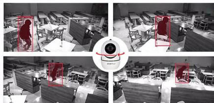
When camera detected the movement of Object from horizontal and vertical direction, will automatically capture its trajectory and push alarm or video to your phone.
