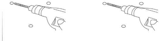
3. Fixed the bracket using three ST4\*35 screws and make sure the installation points are fixed securely.
