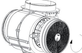
A detailed technical drawing of a cylindrical ventilation duct. A black mesh-like activated carbon filter is shown being inserted into the duct's interior. A curved arrow at the bottom right indicates the direction of rotation for securing the filter in place. |
