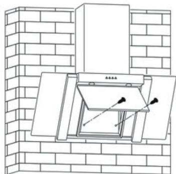
Fix the lower chimney with two 4 x 8 mm screws.
