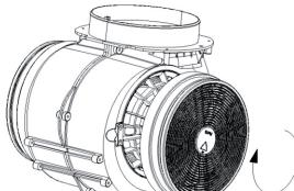
A diagram of a circular fan with a carbon filter attached to its front. A curved arrow indicates the rotation of the fan.                                                                                                                                                |
