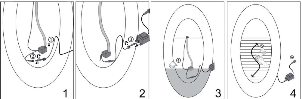
The fountain has been wired-up by the manufacturer. You can usually leave out the first two steps when operating the appliance for the first time.
