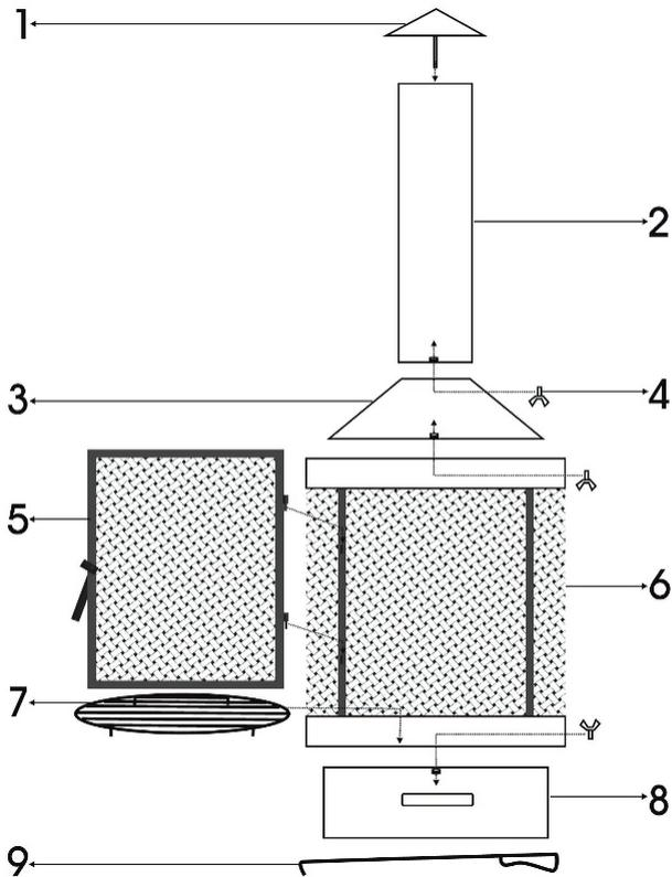
1. Connect the flue (2) to the cover (3) using the bolts (4).
