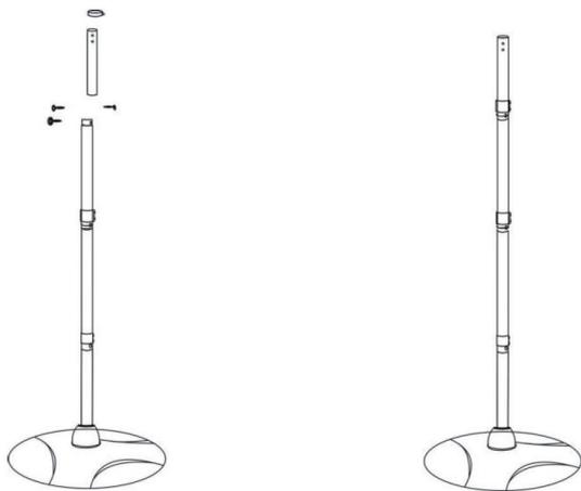
Use same method as step 3 to fix top tube and put third cord support onto the top tube.
