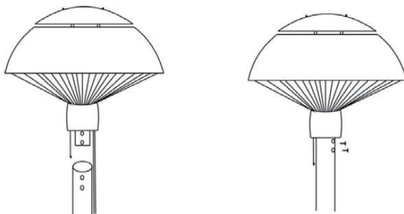
Fix the heater head with top tube by 2 pcs 4\*12 mm screws.
