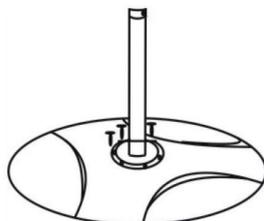
Fix the bottom tube to the base by using 4 pcs 6\*35 mm screws.
