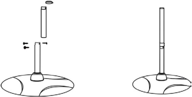
Fix the bottom tube and second tube by 3 pcs 5\*6 mm screws and put first cord support onto the second tube.
