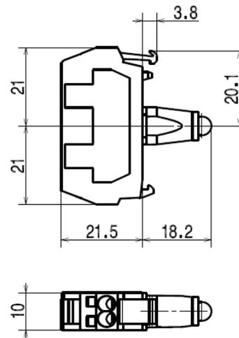
Blocs led raccordement faston
