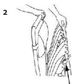
To release the locking system lift lever on both sides of the chair.
