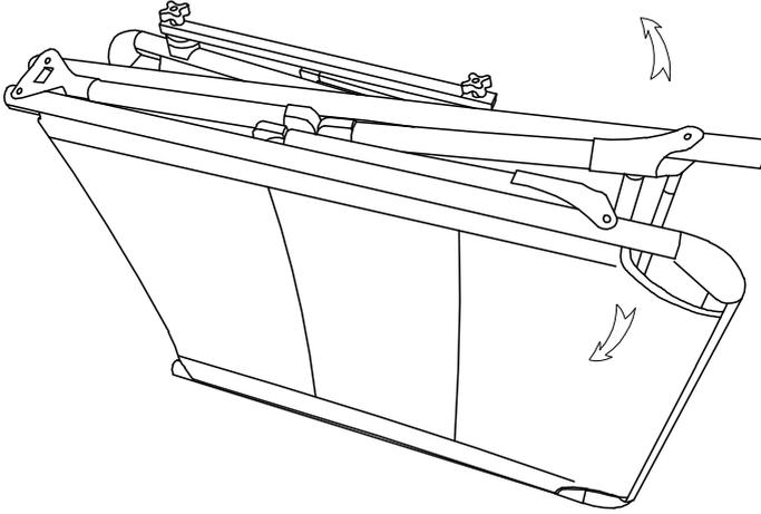
2. Erect the legs. The middle leg must engage. The outer legs must rest on the tube. Check for stability.
