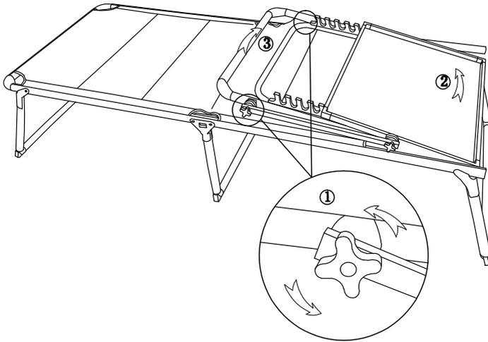
4. Adjust the position of the roof using the hand screws.
