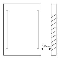
Ensure the sensor are positioned at least 150mm away from any solid surface including walls.
