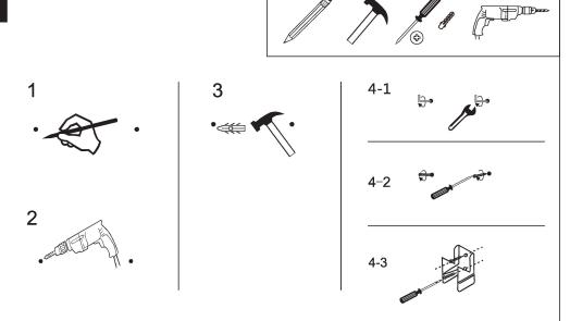
Measure the distance between the two brackets, mark the distance on the wall, check the marks are level, drill the holes, insert the wall plugs and fix according to 4-1, 4-2 or 4-3
