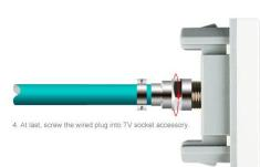
4. At last, screw the wired plug into TV socket accessory
