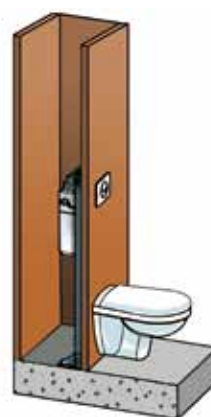
Installation en gaine technique
