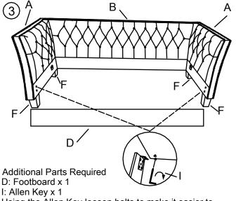
Using the Allen Key loosen bolts to make it easier to position the Footboard in place. Tighten bolts using Allen Key
