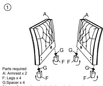
Place a Spacer through the bolt on the Leg and screw in a clockwise direction on the bottom of the Armrest. Repeat this process on all 4 Legs.
