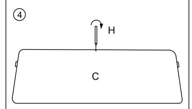
Parts Required H: Middle Leg × 1 Clockwise from the specified position
