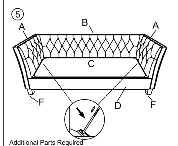
C: Seat Base x 1 Locate the metal clips on the Seat Base and lower into position as illustrated above.
