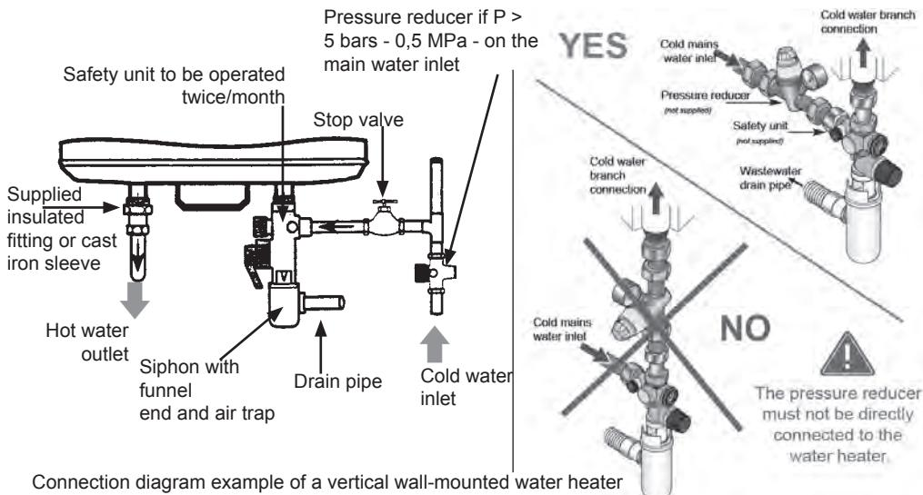
Connection diagram example of a vertical wall-mounted water heater
