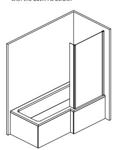
From the inside of the bath screen make a pencil mark on the wall profile approximately 100mm from the top and the bottom.
