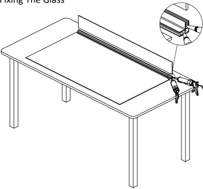
Lay the large panel (4) on a clean flat surface with the corner post (1) facing upwards. In both corner post slots, apply a small bead of silicone along the length of the channel stopping 5mm short of either end and insert the glass panels (4&5).
