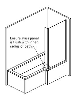
Slide the wall profile (2) onto the screen. Sit the screen onto the bath and adjust so the short glass panel butts upto the inside radius of the bath. Mark the position of the wall profile (2) with a pencil.
