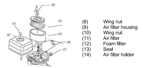
The air filter should be regularly checked and if necessary, cleaned or replaced.
