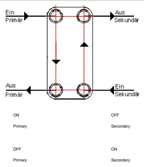
Before commissioning it is necessary to compare the operating data with the manufacturer's indications with regard to their agreement. Moreover, all screw connections have to be checked. The pumps that are providing the plate heat exchanger must be equipped with shut-off valves. The pumps must not suck in air in order to exclude possible malfunctions caused by strokes of water. During the filling of the system, the plate heat exchanger has to be ventilated in order to achieve fully performance.
