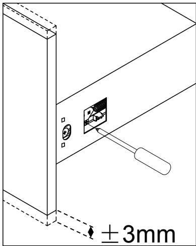
Please use the knobs on both sides of the drawer to adjust its height (up and down) in order to avoid friction with the upper and lower parts.
