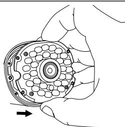
Remove the electronic card by pulling it carefully.
