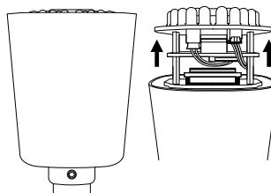
Insert a micro SDHC card into the slot without disconnecting the camera cables and connectors.
