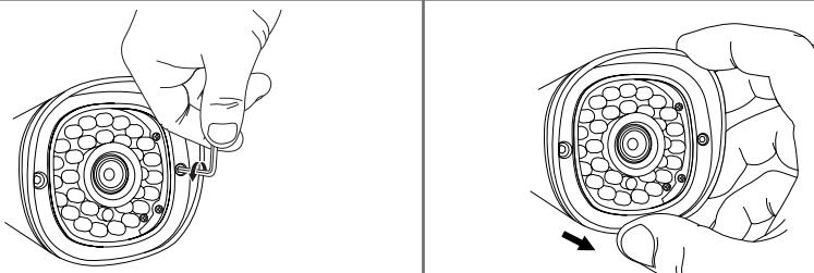
Remove the 4 screws around the electronic card. Warning: do not remove the 4 inside screws.
