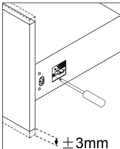
Please use the knobs on both sides of the drawer to adjust its height (up and down) in order to avoid friction with the upper and lower parts.
