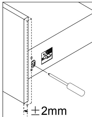
Please use the screw on the right side of the drawer to adjust it horizontally (left and right) in order to avoid friction with the side parts.
