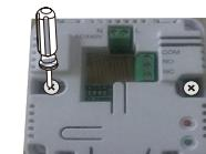
1. Open the receiver with screwdriver
