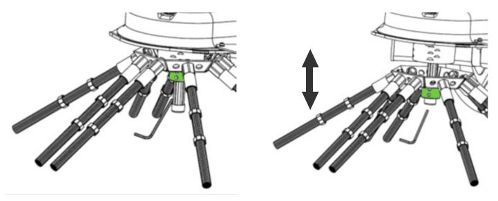
Make sure to adjust the protection frame upwards too as the brushes get worn and when the brush head is adjusted down. Or else the rubber cover will be damaged.
