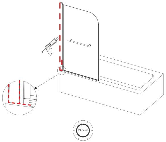
Allow 24 hours for silicone to dry before use. Silicone on the outside edge only, NOT THE INSIDE
