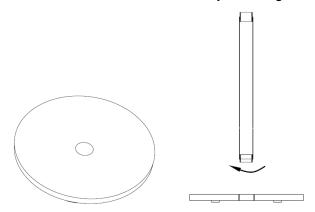
Step 2: Feed the Power Cord through the Base and the Bottom Tube, and pull through around 1.8m of cable.
