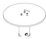
Step 1: Fix the Heater Pole on the base by using the provided 3PCS of M6 \* 12mm screws.
