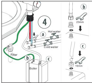
4. Slide the Gasket and retaining ring onto the threaded tube and tighten firmly.
