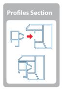
From inside the shower compartment, insert, interlocking, the attachment door profile in the left side profile. Exercise, top to bottom, the pressure needed to hear the insert click. Proceed, then, for the entire length of the side profile.
