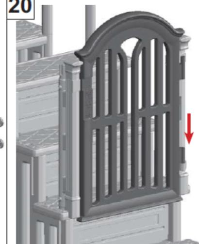
INSÉREZ LES POTEAUX DE PENTURE AVEC LA PORTE ATTACHÉE
