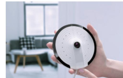
Press and hold the Configuration Button on the side for 5 seconds, and you will hear a tone which indicates that the UFO has switched to the WiFi configuration mode.
