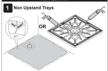
Install the shower tray on a bed of sand and cement or silicone sealant
