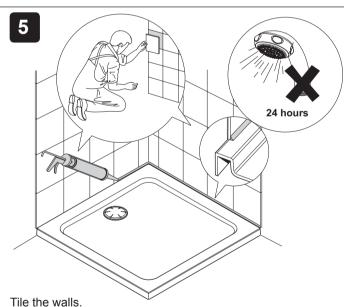
Apply silicone sealant in accordance with the manufacturer's instructions to seal the shower tray to the tiled wall surface.
