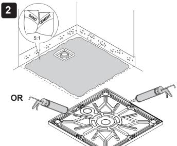
Install the shower tray on a bed of sand and cement or silicone sealant.
