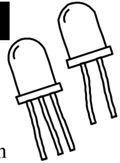
Bicolour LEDs are automatically identified. If your LED has 3 leads then ensure they are all connected, in any order.
