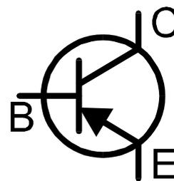
Bipolar Junction Transistors are available in two main types, NPN and PNP. In this example, the unit has detected a Silicon PNP transistor.
