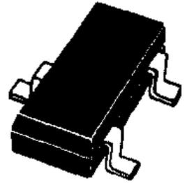
The *Atlas DCA* will intelligently identify popular types of three terminal diode networks. For three terminal devices such as SOT-23 diode networks, the three test clips must all be connected, any way round. The instrument will identify the type of diode network and then display information regarding each detected diode in sequence. The following types of diode networks are automatically recognised by the *Atlas DCA*:
