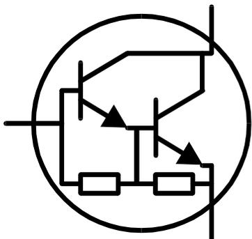
The *Atlas DCA* can detect the resistor shunt if it has a resistance of typically less than 60k $\Omega$ .
