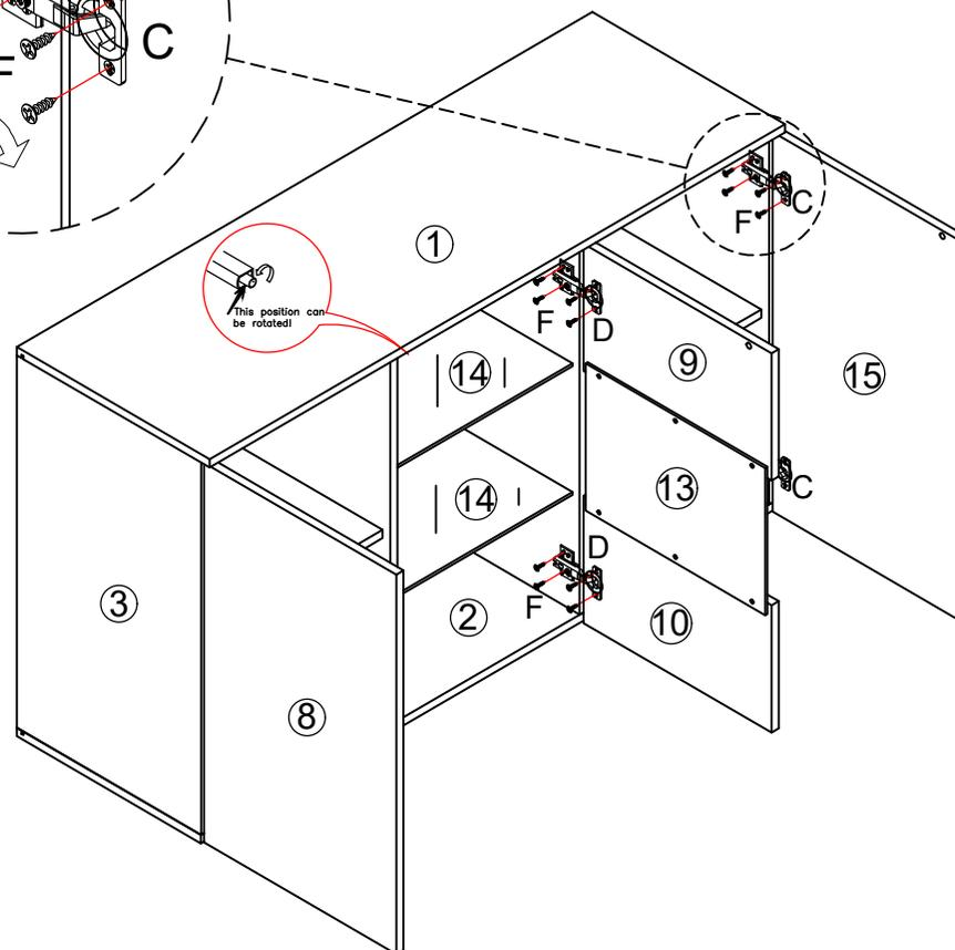
(EN) Piece number 13 is covered by an adhesive that must be removed.
