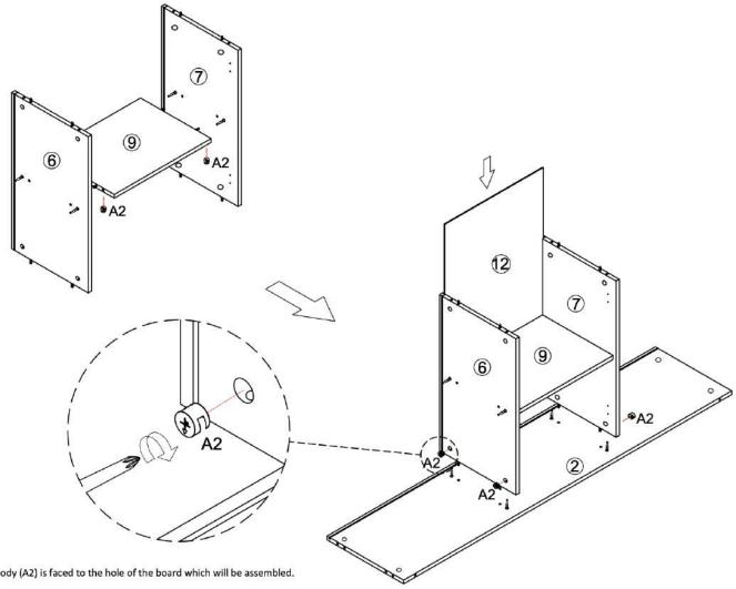
Make sure that the arrow on the minifix body (A2) is faced to the hole of the board which will be assembled.
