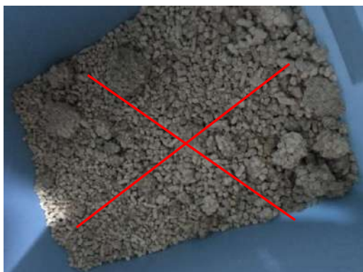
Agglomeration of poor-quality pellets
