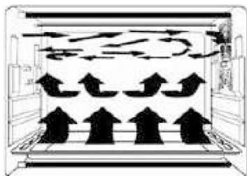
Due to the fan located on the side of the oven cavity the hot air circulates throughout the entire oven. The heat is therefore better distributed and cooking is more even.
