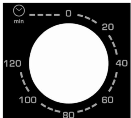
Adjust the timer to the appropriate cooking duration (in minutes) for the dish you are going to cook by turning it clockwise.
