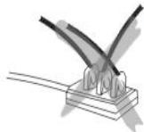
The oven must be connected to a suitable electrical socket. Make sure the plug is completely in the socket. Otherwise it could overheat. Do not use a lighting socket. Never connect several plugs to the same socket.
