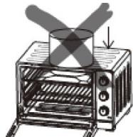
Do not put anything between the base of the oven and the surface on which it stands. Anything placed under the oven could be burnt. Do not place anything on the oven when it is operation because the heat could possibly distort, crack or damage it.
