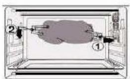
Insert the rotisserie forks in the rotisserie orifice and then place the drip pan under the rotisserie
