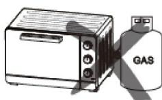
When in use never place the machine near a gas burner, a source of high heat or an electric fan, etc. This could damage the temperature control.
