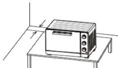
If the oven is placed too close to a wall this could be burnt or stained. Make sure that curtains, etc. are not in contact with the oven.
