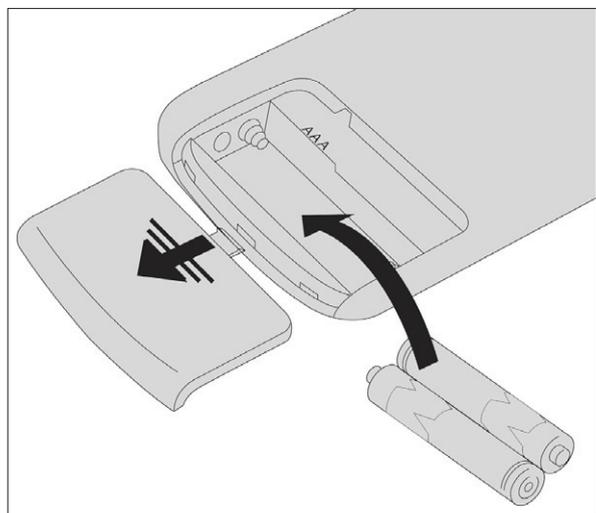
**SI LA TÉLÉCOMMANDE EST ÉTEINTE PAR ABSENCE DE BATTERIES, IL EST POSSIBLE DE COMMANDER LE POËLE PAR LE PANNEAU DE COMMANDES PLACÉ DANS LA PARTIE SUPÉRIEURE DU POËLE. PENDANT L'OPÉRATION DE REMPLACEMENT, PRÊTER ATTENTION À LA POLARITÉ, EN SUIVANT LES SYMBOLES IMPRIMÉS SUR LE COMPARTIMENT INTERNE DE LA TÉLÉCOMMANDE.**
