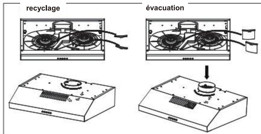
**VÉRIFIER SYSTÉMATIQUEMENT QUE LA OU LES LAMELLE(S) MONTÉE(S) EST(SONT) CORRECTE(S).**
