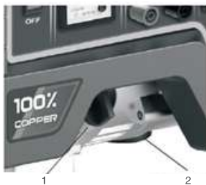
1. Oil filler hole 2. Oil filler cap
