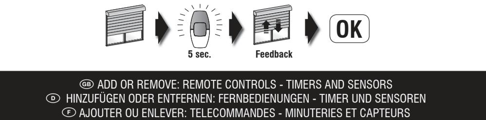
(B) ADD OR REMOVE: REMOTE CONTROLS - TIMERS AND SENSORS - (C) HINZUFÜGEN ODER ENTFERNEN: FERNBEDIENUNGEN - TIMER UND SENSOREN - (F) AJOUTER OU ENLEVER: TELECOMMANDES - MINUTERIES ET CAPTEURS
