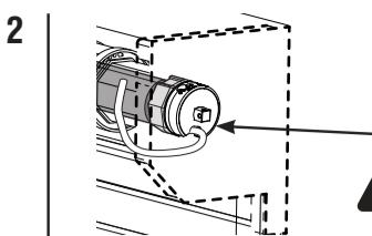
(B) Make sure wires do not get in the way of moving parts.
