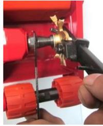
To remove the cutter, use the cutter wrench & spanner
