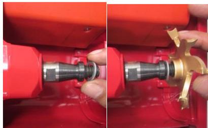
Install Cutter step by step as follows:
