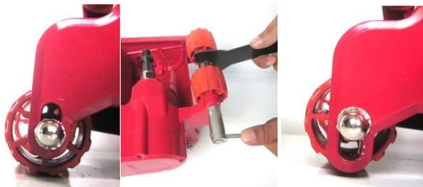
Adjust height of front rollers to control chasing depth
