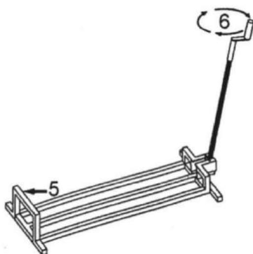
If the mower is leaning please turn the handle to lower the mower on the ground. Place the mower correctly and start the lifting again.
