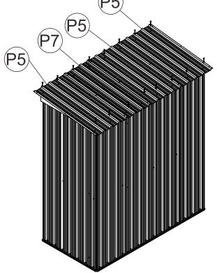
Assemble the roof flashing (15)(16)(17) with roof panels. Secure with (F1) screws with washers. Then place 4 piece of top corner(GC) on the roof joints and secure with screws with washers.
