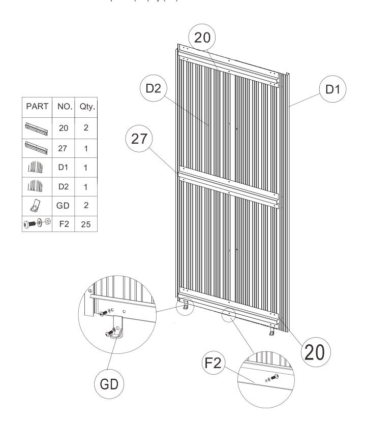
**Note**: the door handle(GB) the third hole need fix with door panel(D2) and door bar (27).
