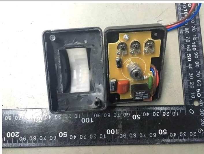
Photo 24 Description: Open view of sensor for KS901
