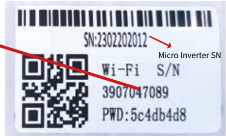
Micro Inverter SN: 2302202012 Built-in datalogger :3907047089
