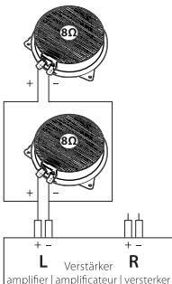
Connection of 2 **bassPUMP®** each channel to 4 ohm capable amplifier speaker output up to 100W rms.
