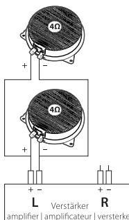
Connection of 2 **bassPUMP®** each channel to 2 ohm capable amplifier speaker output up to 100W rms.
