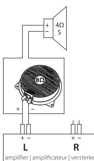
Connection of 1 **bassPUMP®** plus S=front or rear speaker system each channel to 4 ohm capable amplifier speaker output up to 100W rms.
