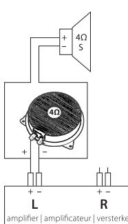
Connection of 1 **bassPUMP®** plus S=front or rear speaker system each channel to 2 ohm capable amplifier speaker output up to 100W rms.
