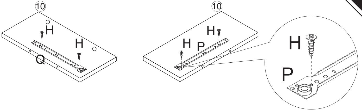
**EN** Please find the exact hole for installation, otherwise it will be misaligned. The screws on the drawer slide must be leveled , otherwise it will affect the smoothness of the d rawer.
