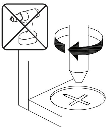
**EN**\_Turn cam lock clockwise to tighten.
