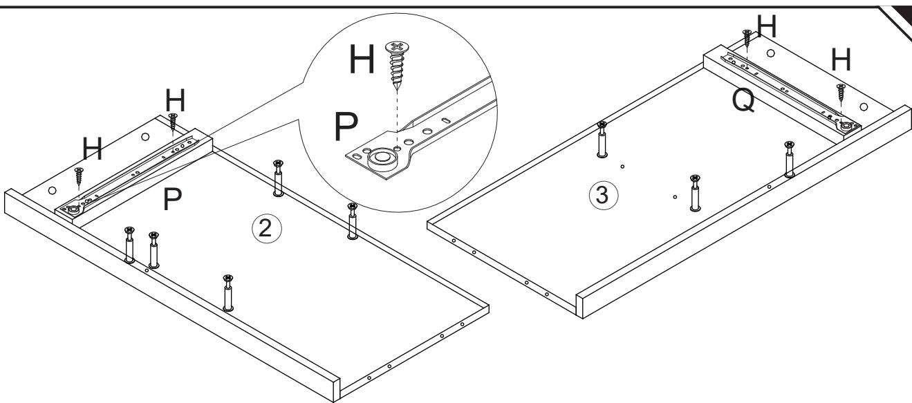
**EN** Please find the exact hole for installation, otherwise it will be misaligned. The screws on the drawer slide must be leveled , otherwise it will affect the smoothness of the d rawer.
