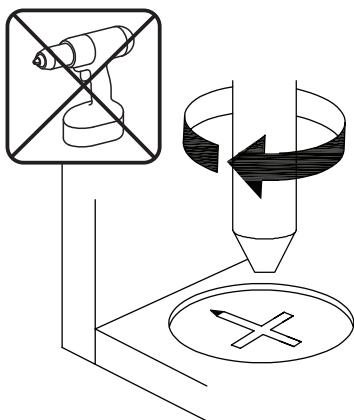
**EN**\_Turn cam lock clockwise to tighten.
