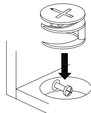
**EN**\_Quickfit head should be in the centre of the cam lock when the two panels are joined.
